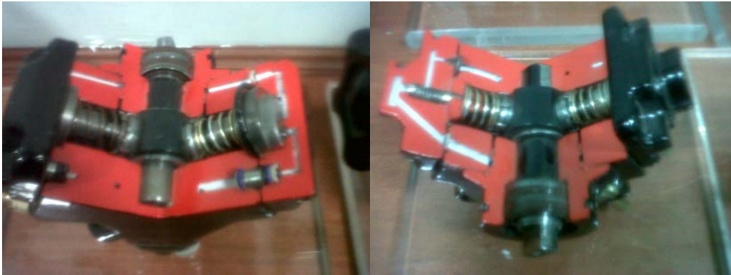
Fig 16 : Cut section view of high pressure pump
