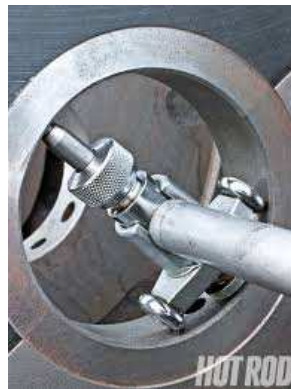
Fig.22 Using bore gauge showing measuring sled
