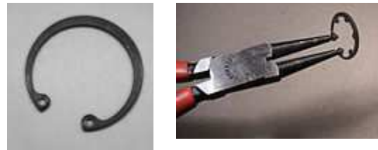
Fig-21 Circlip and circlip plier
