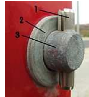
Fig-23 slotted spring pin (1) and washer (2) used to secure a shaft (3)
