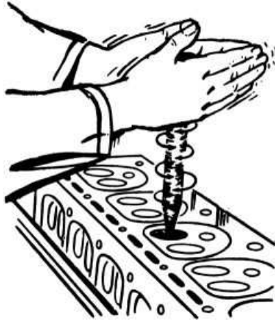
Fig 10 : Valve Lapping process
