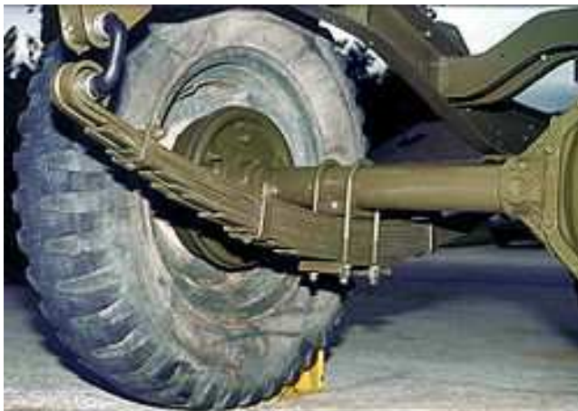
Fig 2: Leaf spring fitted in a vehicle
