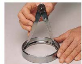
Checking inside groove.
