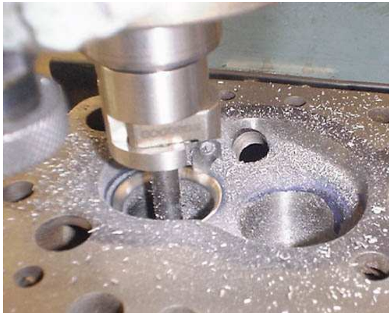
Fig 9 : Seat Cutting operation
