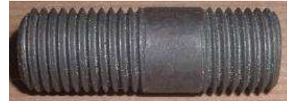
Fig-131 screw-in type stud
