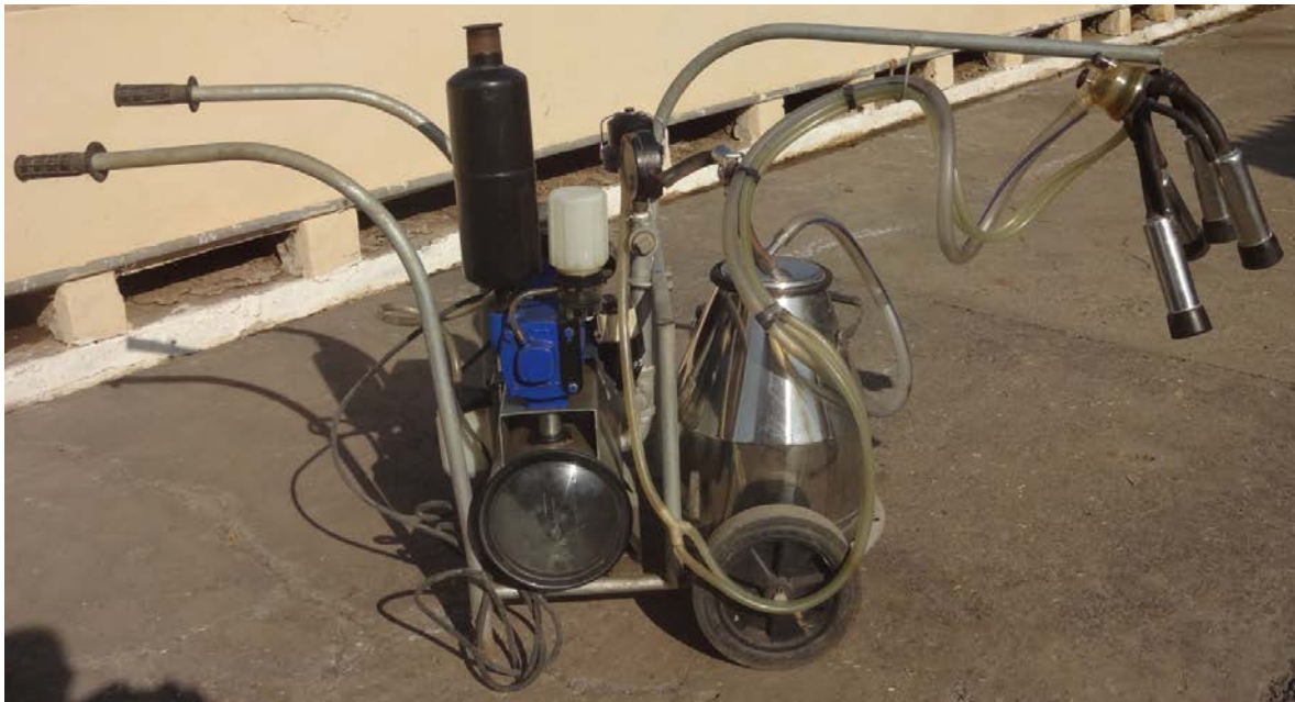
Figure 2.13: Mobile bucket type milking machine suitable for medium size dairy farms
