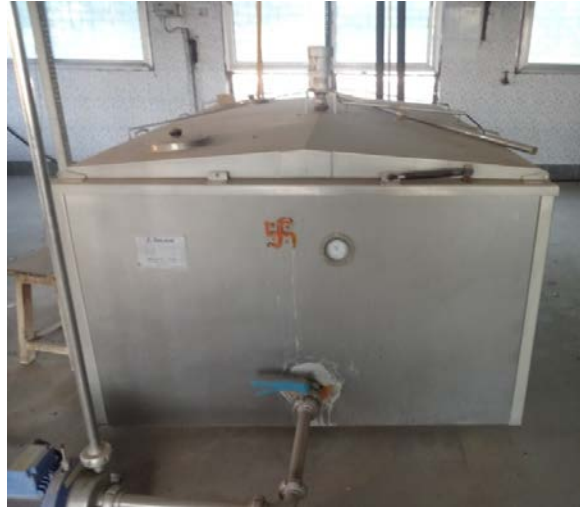
Figure 2.7: Milk chilling tank of 1000 litres capacity
